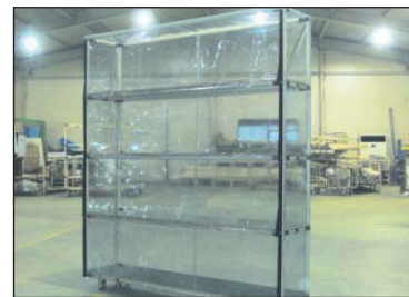
24. MOVING CART FOR PREVENTING DIRT
