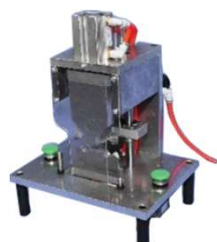
Đồ gá cắt phoi đúc – J05 Burr cutting Jig for casting part
